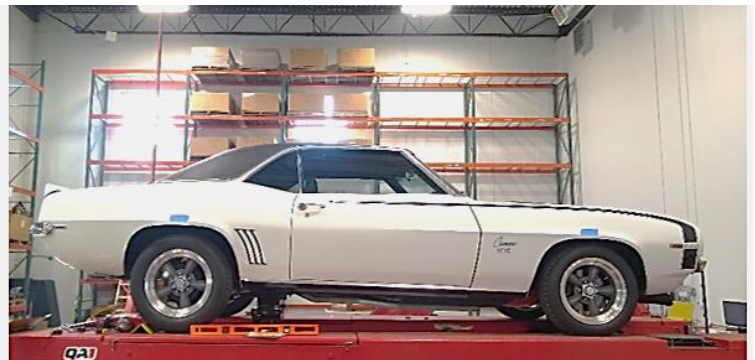
As shown: 16x8 American Racing, 4.07" Back space. Front: 225/50/16 Rear: 255/60/16
