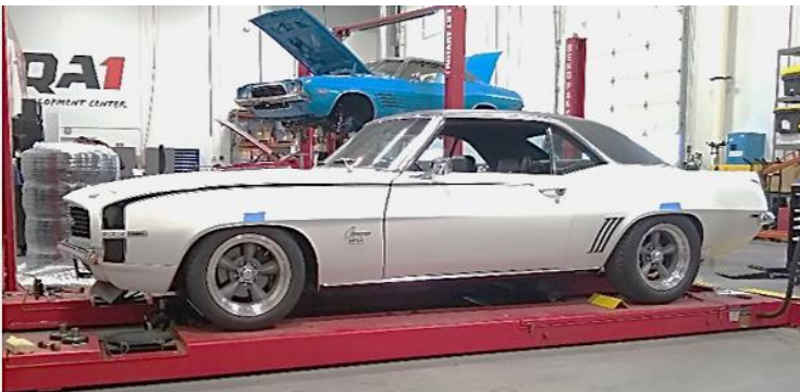
As shown: 16x8 American Racing, 4.07" Back space. Front: 225/50/16 Rear: 255/60/16
